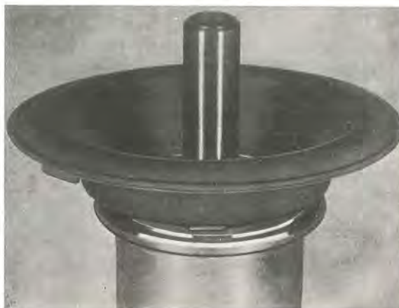
Fig. 2-70. Diaphragm in air valve
