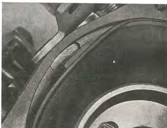
Fig. 2-71. Diaphragm fitted in main carburettor body
