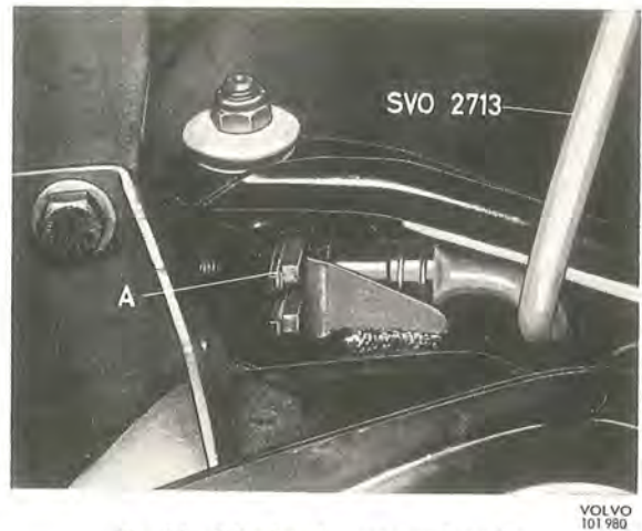
Fig. 6-8. Adjusting the caster and camber A=Shims
