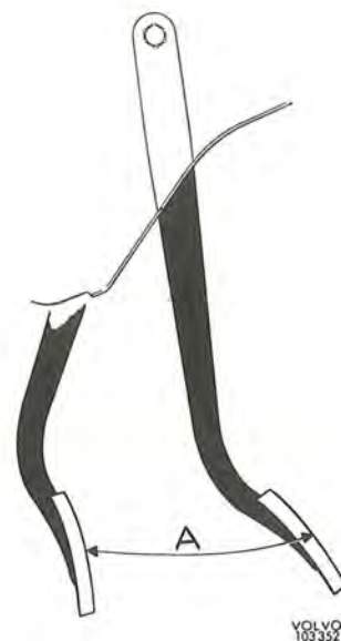
Fig. 5-62. Pedal travel A=approx. 152 mm (6")
