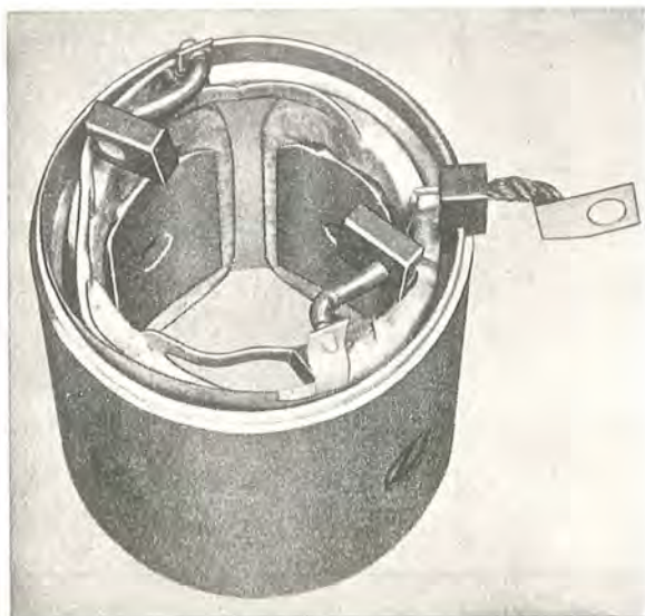
Fig. 3-43. Stator with soldered brushes
