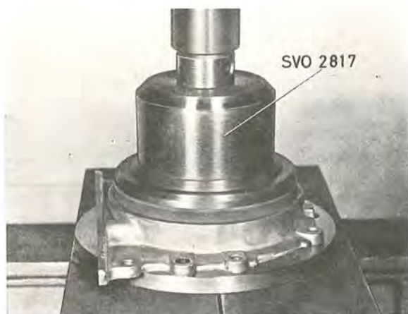
Fig. 2-28. Fitting oil seal
