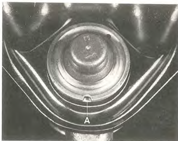
Fig. 6-22. Location of ball joint in upper wishbone
