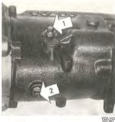
Fig. 1-3. Gearbox 1. Filler plug 2. Drain plug
