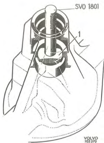
Fig. 4-78. Removing the rear pinion bearing race 1. Removing drift SVO 2843
