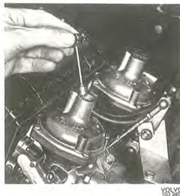
Fig. 1-2. Checking the oil level in centre spindle
