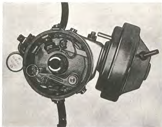
Fig. 3-56. Recess for adjusting the contact breaker
