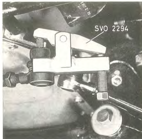
Fig. 6-19. Removing the steering rod
