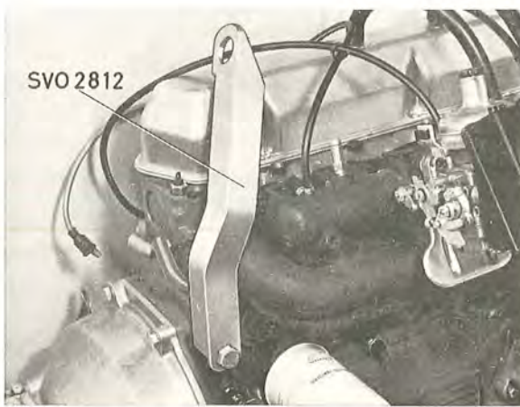
Fig. 2-10. Lifting arm SVO 2812 on rear end of engine
