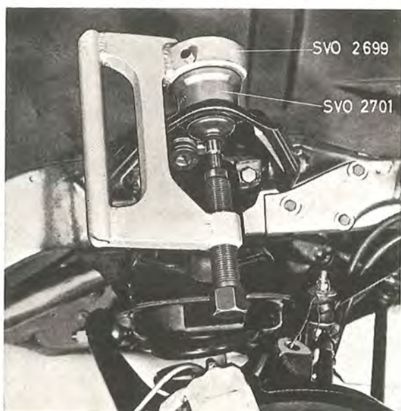
Fig. 6-21. Removing the ball joint, upper wishbone
