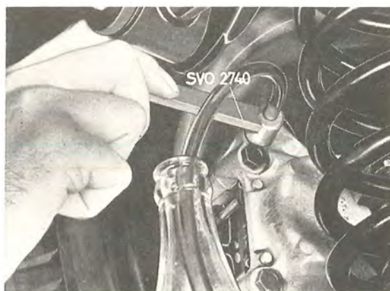
Fig. 5-66. Venting the left rear wheel brake unit
