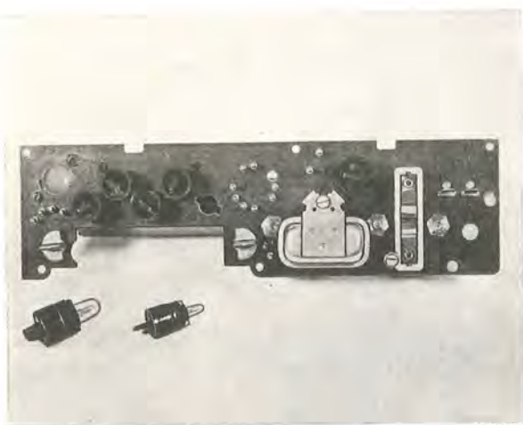
Fig. 9-4. Instrument base plate, reverse side, with warning lamp and instrument lighting lamp
