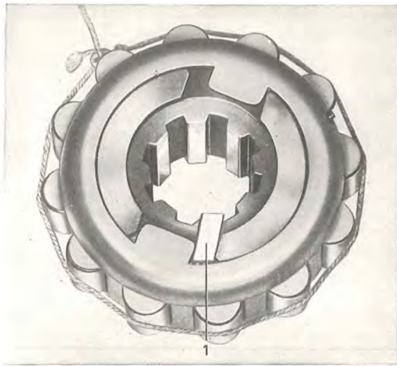
Fig. 4-52. Assembling the uni-directional clutch, II 1. Key
