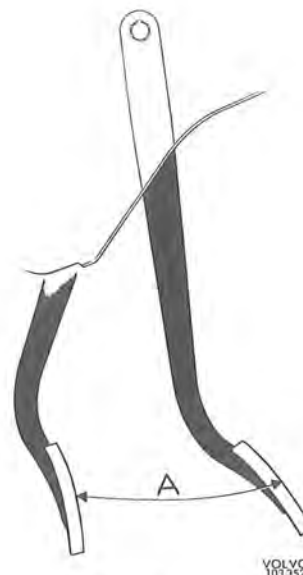
Fig. 5-62. Pedal travel A=approx. 152 mm (6")
