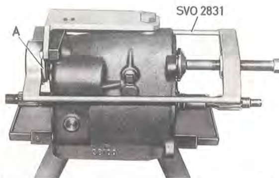
Fig. 4-30. Fitting intermediate shaft bearing A. Insert drift
