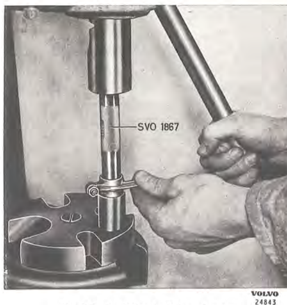
Fig. 2-23. Replacing bush in rocker arm
