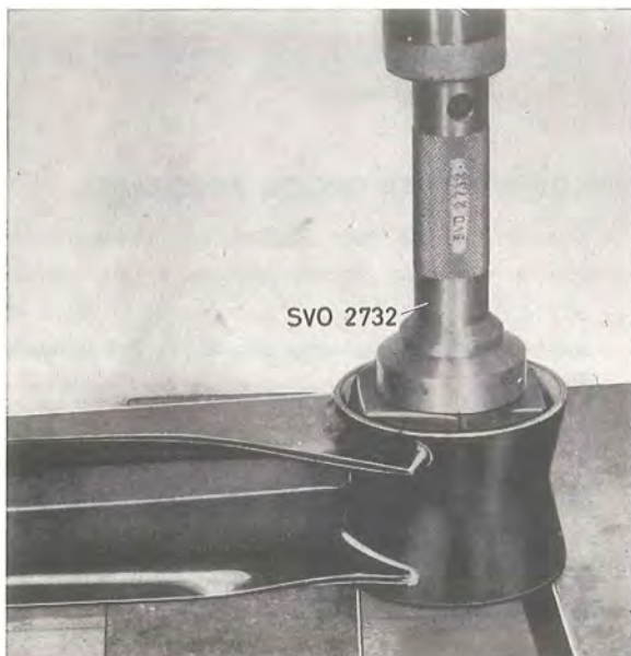
Fig. 7-10. Removing (and fitting) the front bush, support arm
