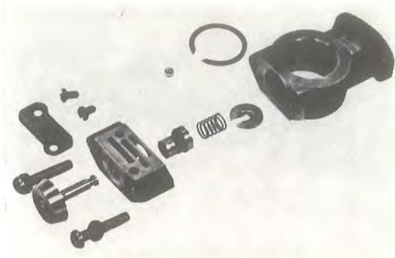
Fig. 4-100. Governor assembly dismantled
