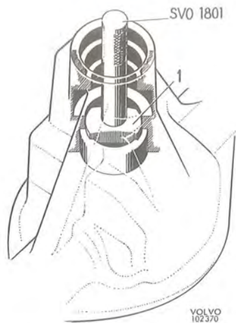
Fig. 4-142. Removing the rear pinion bearing race 1. Removing drift SVO 2843
