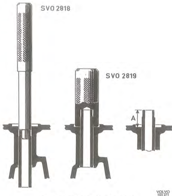
Fig. 2-21. Replacing the valve guides A=17.5 mm (.689")
