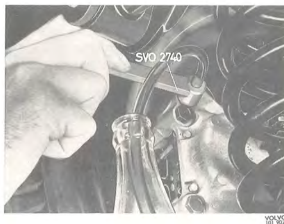
Fig. 5-66. Venting the left rear wheel brake unit
