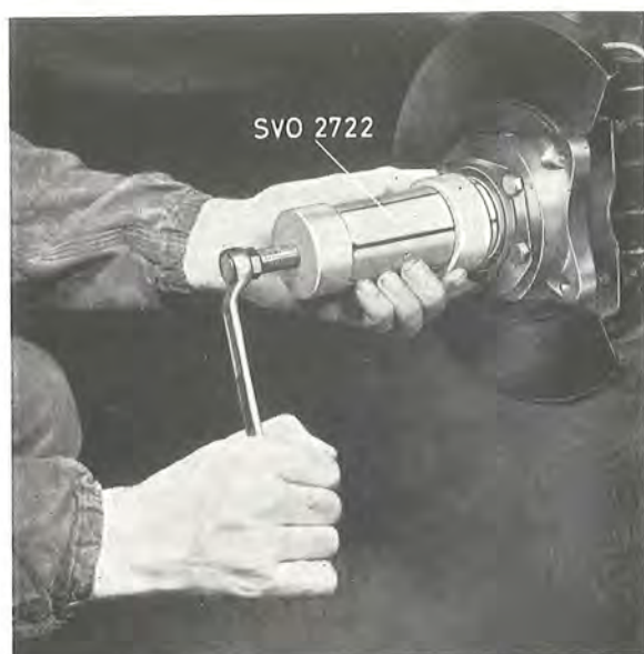
Fig. 7-21. Removing the inner bearing
