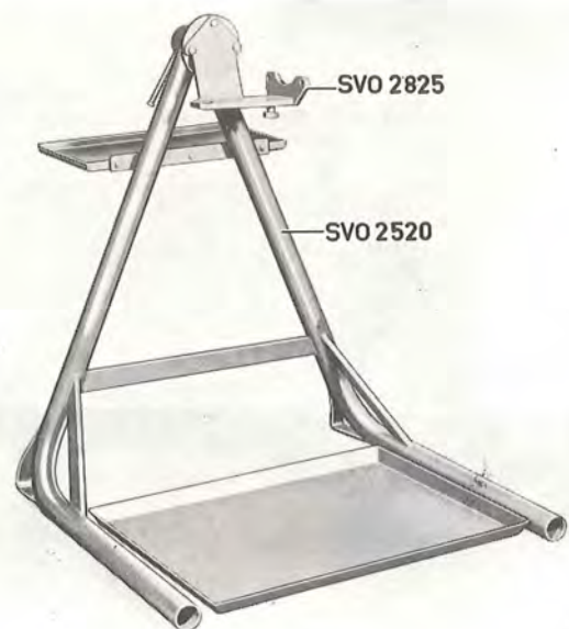
Fig. 4-12. Stand SVO 2520 with fixture SVO 2825
