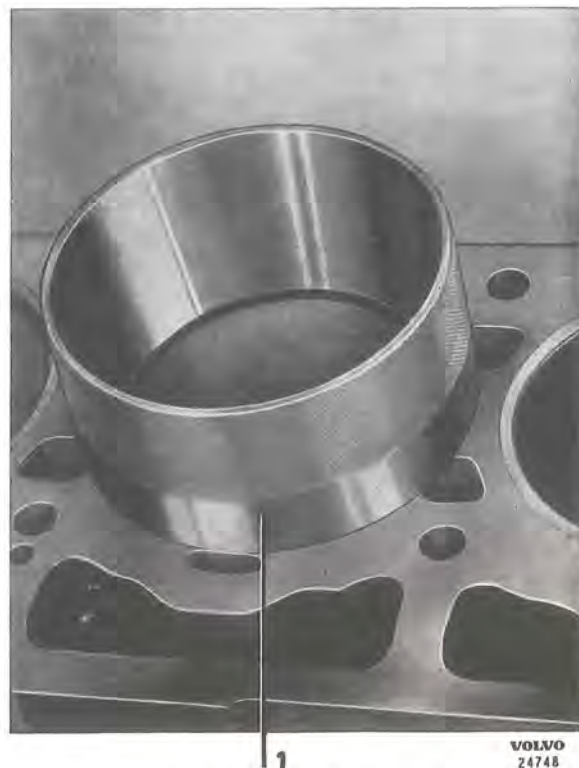
Fig. 2-25. Fitting the piston 1. Fitting ring SVO 2823
