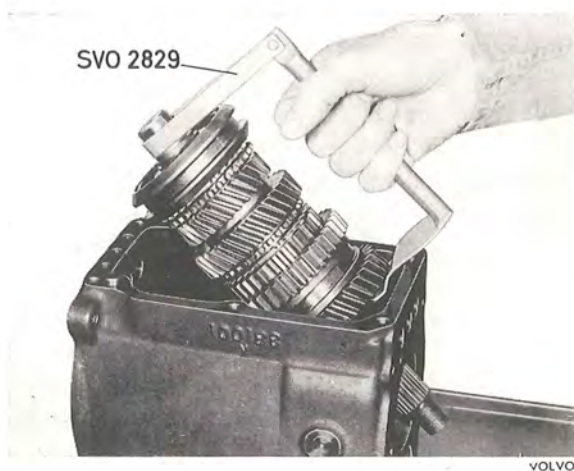
Fig. 4-22. Lifting out the mainshaft
