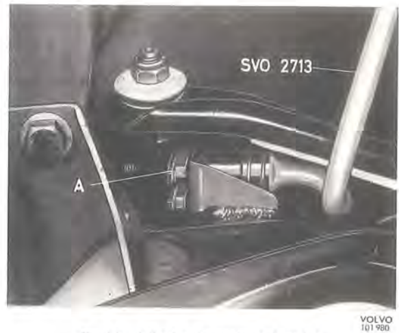
Fig. 6-8. Adjusting the caster and camber A=Shims
