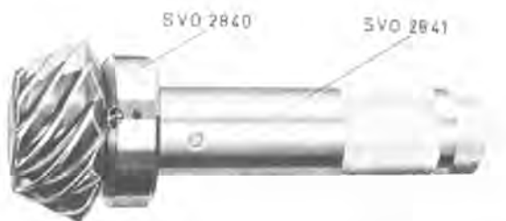
Fig. 4-150. Adjusting ring and tool for pinion location
