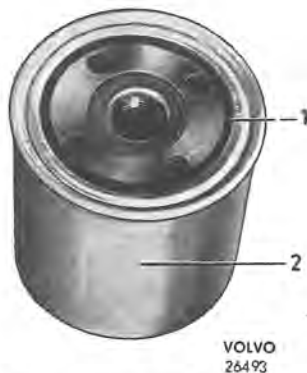
Fig. 2-49. Oil filter ready for fitting 1. Gasket (oiled) 2. Filter
