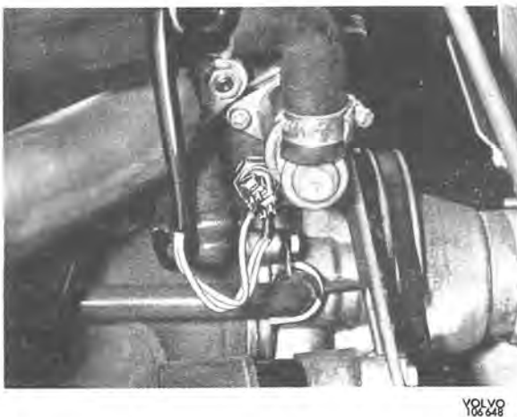
Fig. 2-119. Thermal timer installed
