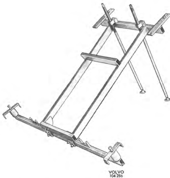
Fig. 8-2. SVO 2777 Fixture for replacing side-members
