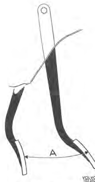
Fig. 5-62. Pedal travel A=approx. 152 mm (6")
