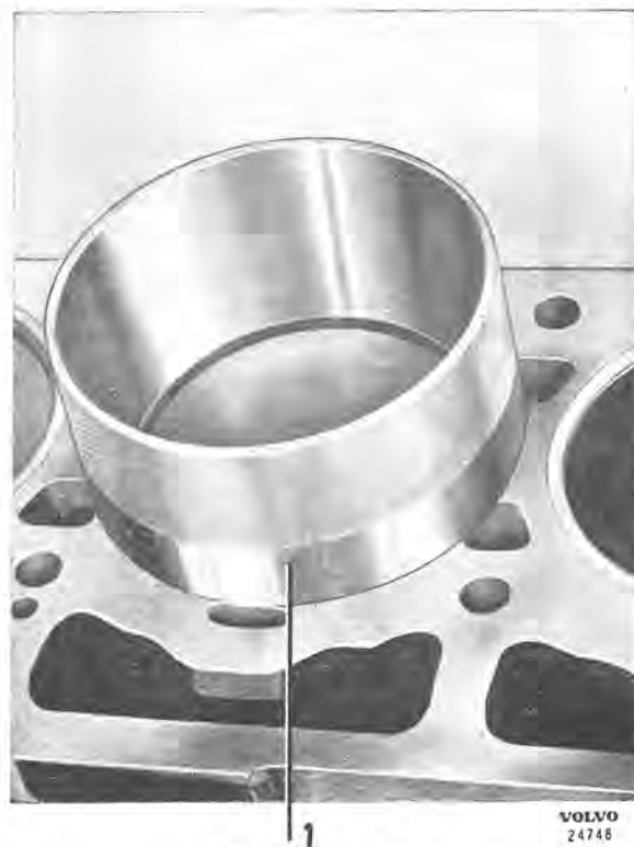
Fig. 2-31. Fitting piston 1. Fitting ring SVO 2823
