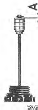
Fig. 2-93. Damper plunger clearance
