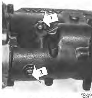
Fig. 1-3. Gearbox 1. Filler plug 2. Drain plug
