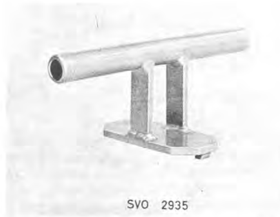
Fig. 3-98. Special tool for removing and fitting tank armature
