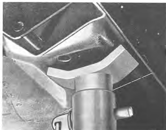
Fig. 7-4. Location of axle prop for propping up vehicle rear end
