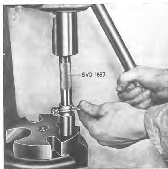
Fig. 2-29. Replacing bush in rocker arm
