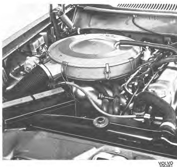
Fig. 2-123. Air cleaner, installed
