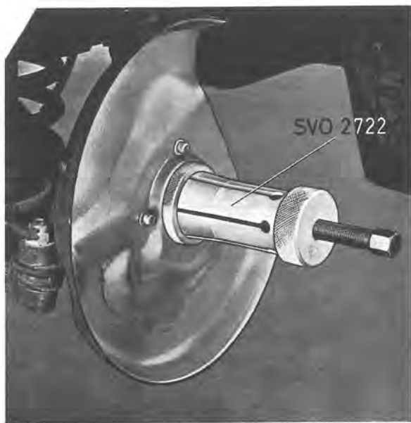
Fig. 7-21. Removing inner bearing
