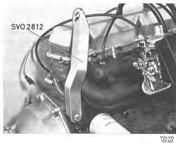
Fig. 2-14. Lifting arm SVO 2812 on rear end of engine
