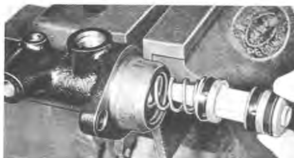
Fig. 5-50. Installing secondary piston
