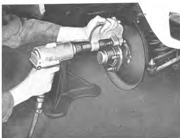
Fig. 7-17. Removing wheel stud
