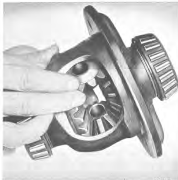
Fig. 4-149. Installing differential gear
