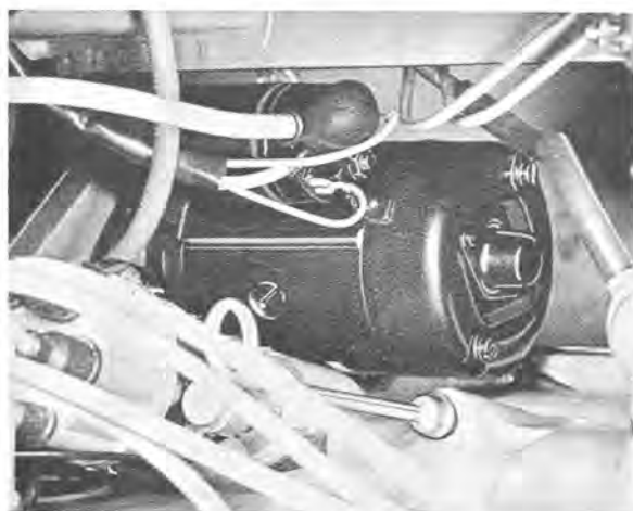
Fig. 3-29. Starter motor installed
