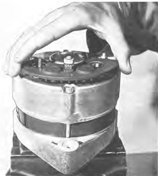
Fig. 3-6. Removing isolation diodes
