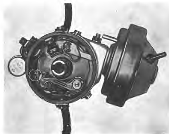
Fig. 3-58. Recess for adjusting ignition contact breaker
