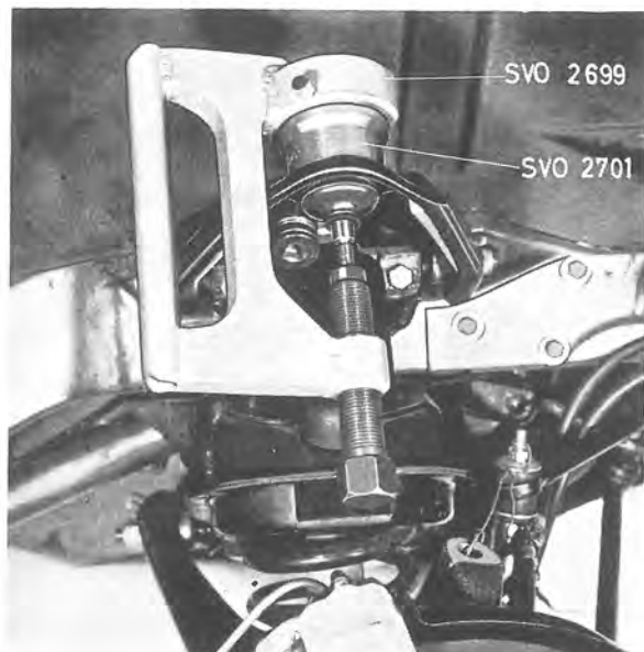
Fig. 6-21. Removing upper ball joint
