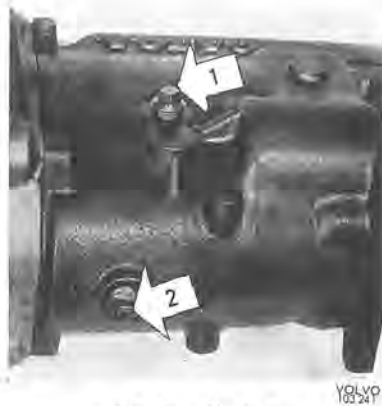
Fig. 1-3. Gearbox 1. Filler plug 2. Drain plug
