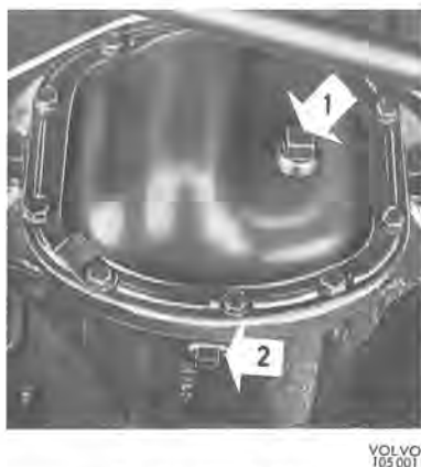
Fig. 1-6. Final drive 1. Filler plug 2. Drain plug
