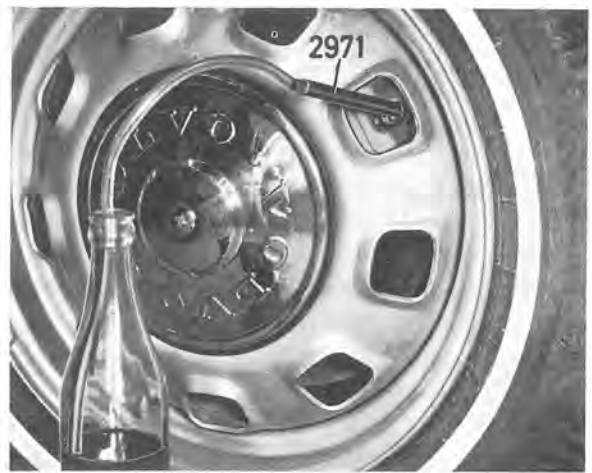
Fig. 5-63. Bleeding front wheel brake unit
