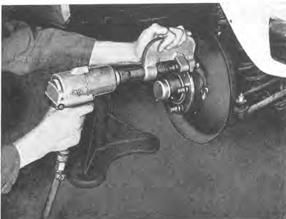
Fig. 7-17. Removing wheel stud
