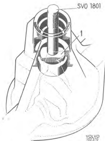
Fig. 4-148. Removing rear pinion bearing race 1. Removing drift 2843
