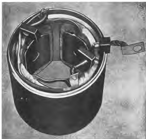
Fig. 3-43. Stator with soldered brushes
