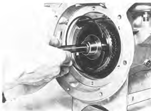
Fig. 4-116. Installation sequence, front clutch snap ring, input shaft and thrust washer
