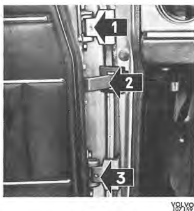
Fig. 1-11. Hinges 1. Hinges, grease 2. Door stop, paraffin wax 3. Hinges, grease
