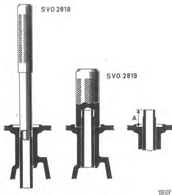
Fig. 2-27. Replacing valve guides A=17.5 mm (0.689")
