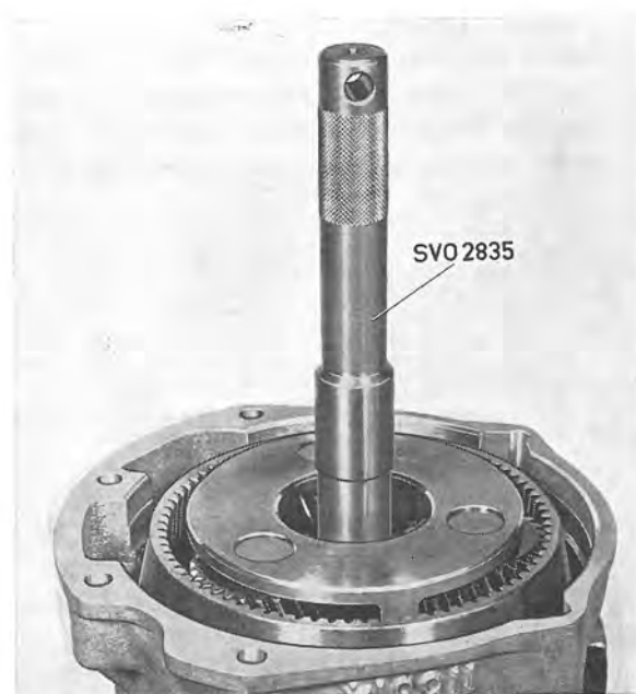
Fig. 4-58. Installing planet gear
