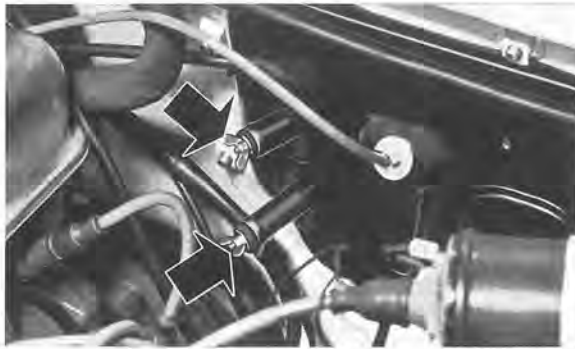
Fig. 8-53. Fitting plugs in heater system connection pipe
