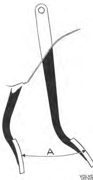
Fig. 5-60. Pedal travel A=approx. 152 mm (6")
