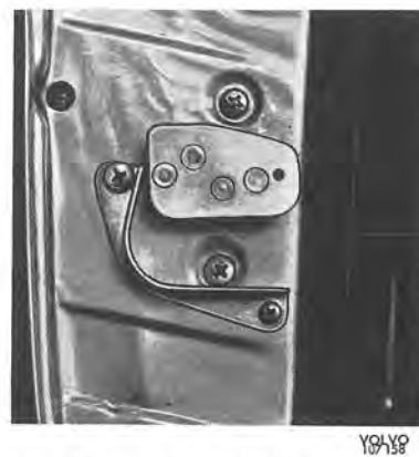
Fig. 1-13. Door lock with guide plate Apply paraffin wax
