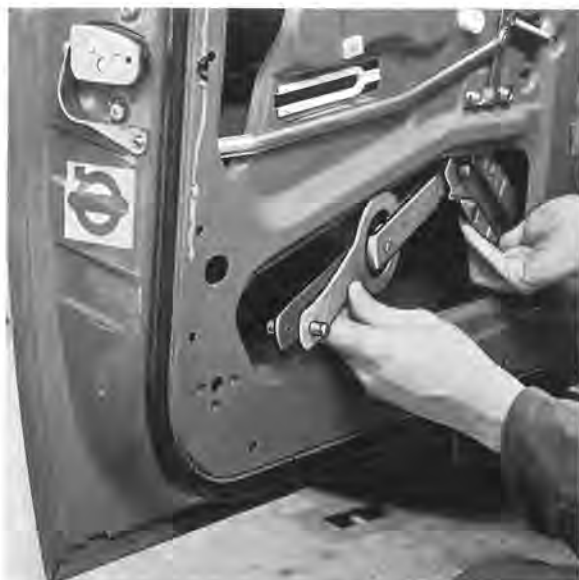
Fig. 8-20. Window mechanism removal
