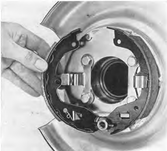
Fig. 5-84. Removing the brake shoes
