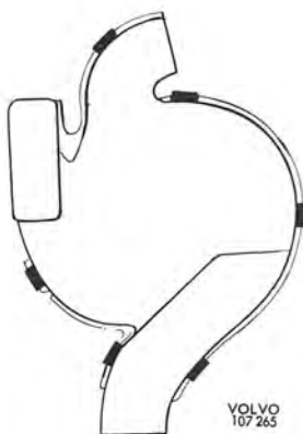
Fig. 8-61. Placing clamps for outer end
