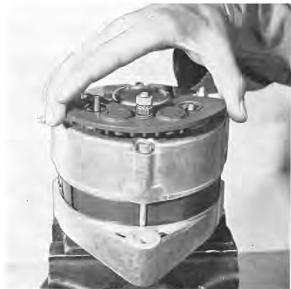
Fig. 3-6. Removing isolation diodes
