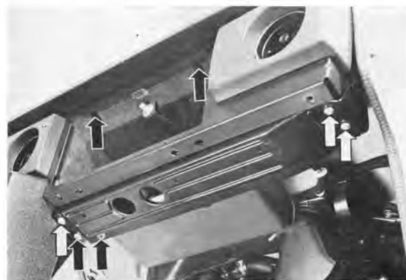
Fig. 8-63. Screw for member and glove locker
