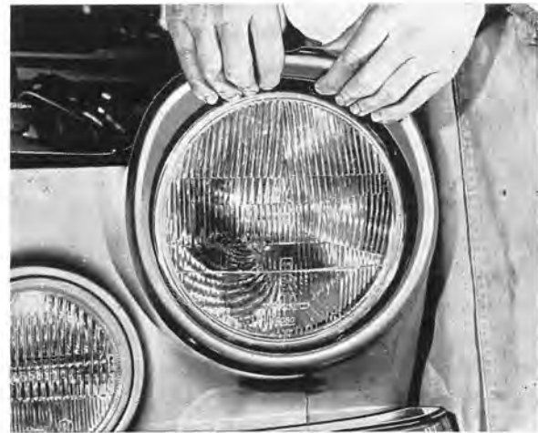
Fig. 3-74. Removing outer rim
