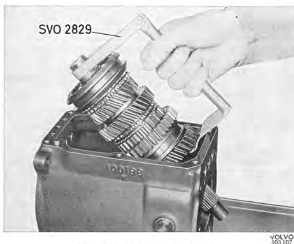
Fig. 4-21. Lifting out mainshaft
