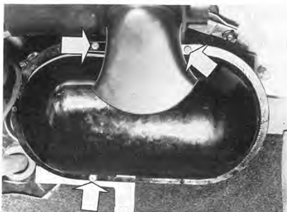
Fig. 8-67. Screws for vacuum tank
