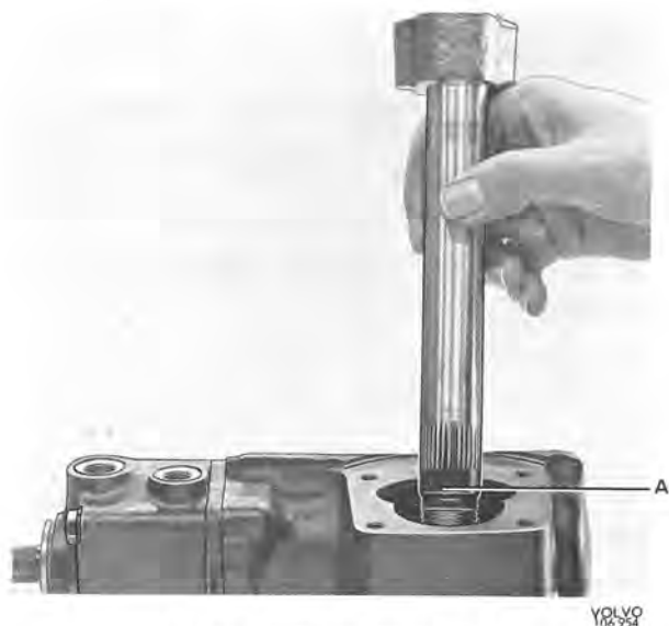
Fig. 6-85. Installing steering shaft
