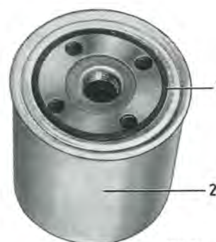
Fig. 2-49. Oil filter ready for fitting 1. Gasket (oiled) 2. Filter
