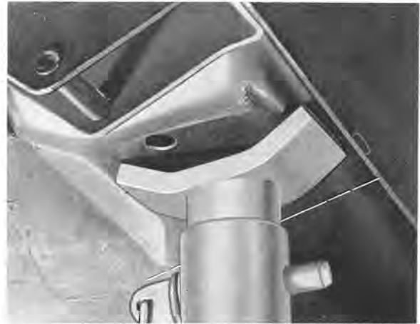
Fig. 7-3. Location of axle prop for propping up vehicle rear end
