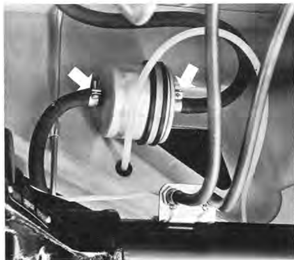
Fig. 2-138. Removing fuel filter
