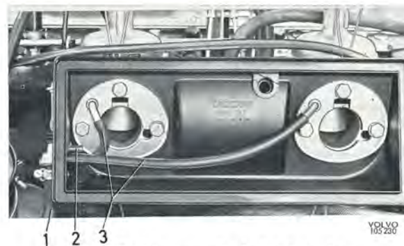
Fig. 2-67. Hose connection for hot start valve
