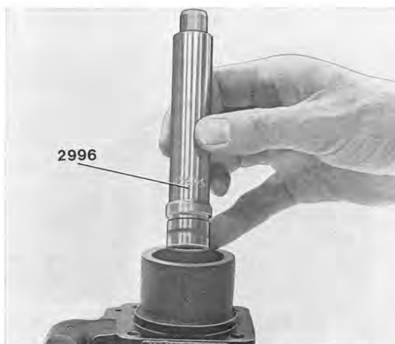
Fig. 6-91. Installing needle bearing
