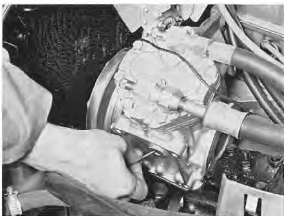
Fig. 8-81. Checking oil level in compressor
