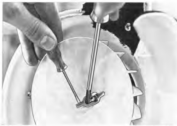
Fig. 8-59. Removing locking for turbine
