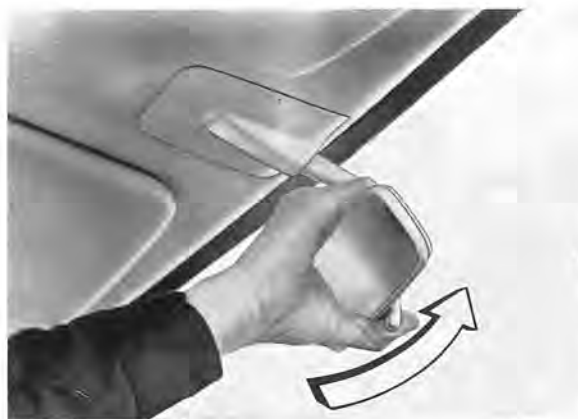
Fig. 8-53. Removing rearview mirror
