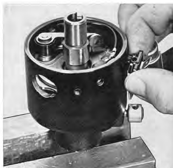
Fig. 3-53. Removing primary connection
