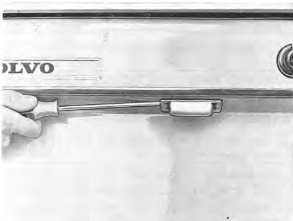
Fig. 3-80. Removing license plate light
