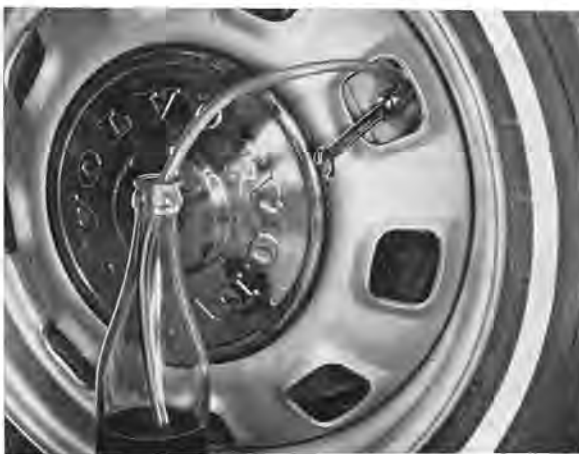
Fig. 5-65. Bleeding front wheel brakes
