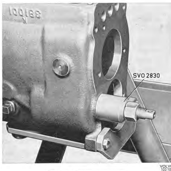
Fig. 4-23. Removing reverse shaft
