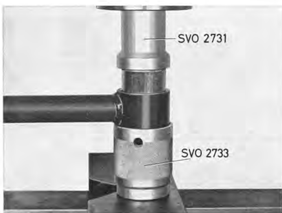
Fig. 7-13. Installing large bush, track bar
