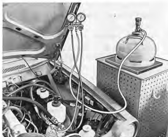
Fig. 8-87. Connecting refrigerant can
