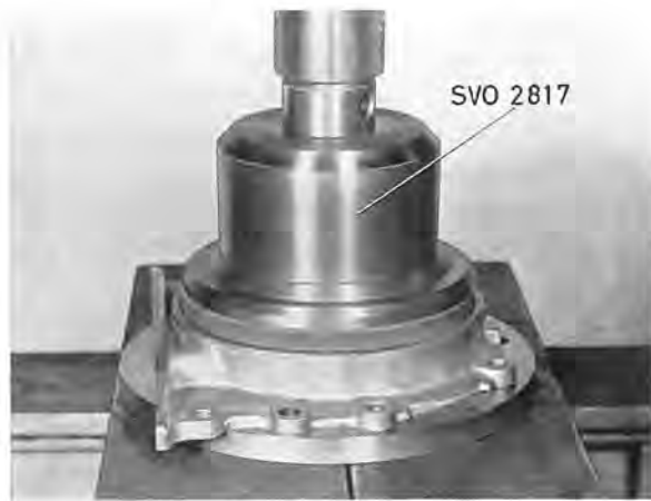
Fig. 2-34. Fitting oil seal
