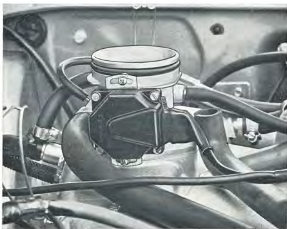
Fig. 2-109. Throttle valve switch installed
