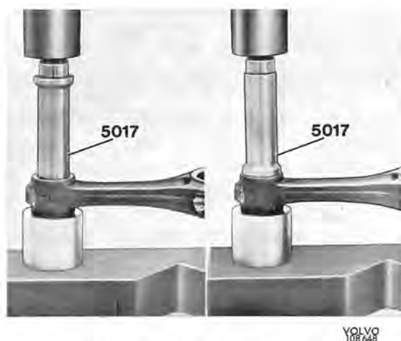
Fig. 2-32. Replacing bush in connecting rod
