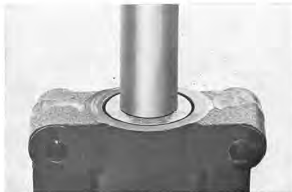
Fig. 6-68. Installing needle bearing
