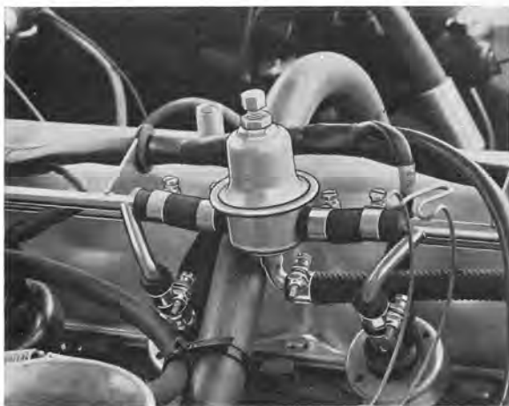
Fig. 2-139. Replacing pressure regulator
