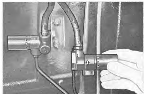
Fig. 5-58. Removing brake valve
