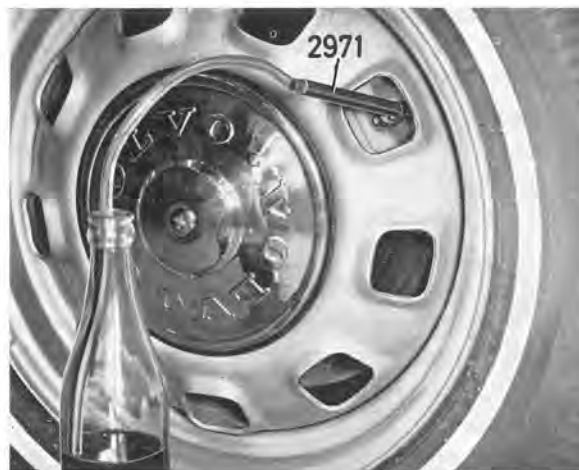
Fig. 5-63. Bleeding front wheel brake unit
