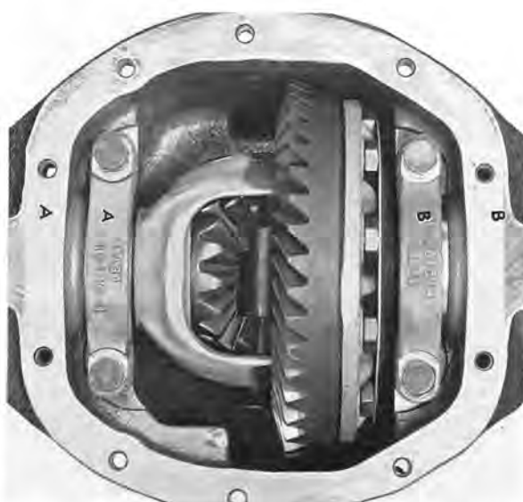
Fig. 4-146. Alignment marking on cap and carrier
