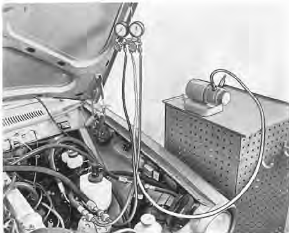
Fig. 8-86. Connecting vacuum pump
