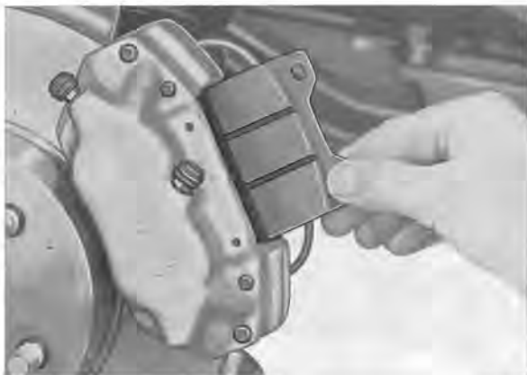
Fig. 5-17. Installing brake pads
