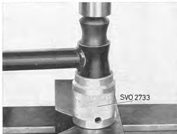
Fig. 7-14. Installing bush, support stay
