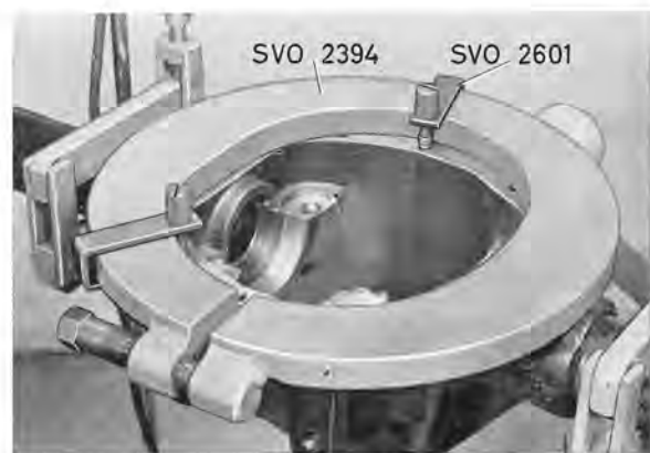
Fig. 4-147. Expanding drive pinion carrier
