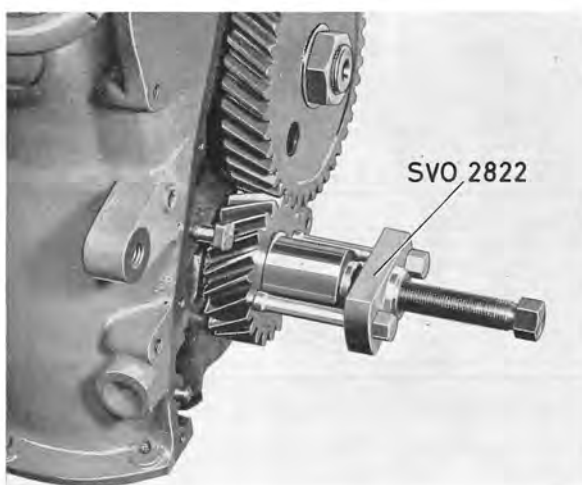
Fig. 2-41. Removing crankshaft gear
