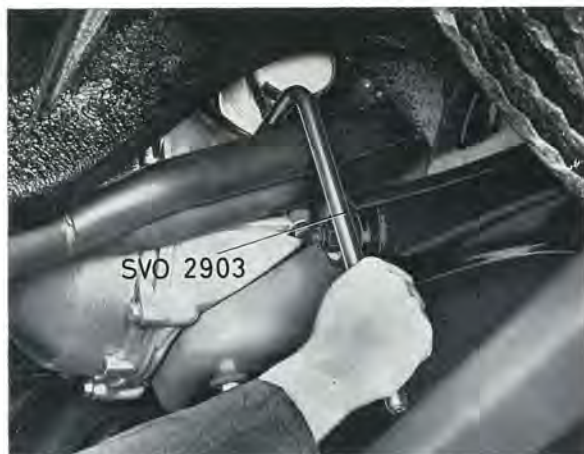
Fig. 2-48. Removing oil filter
