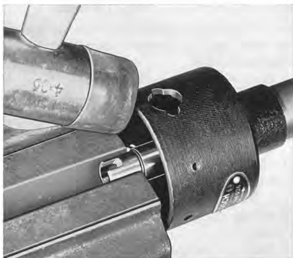
Fig. 3-54. Removing snap ring
