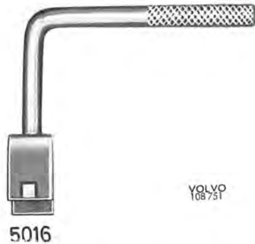
Fig. 3-109. Special tool for removing and installing tank fittings
