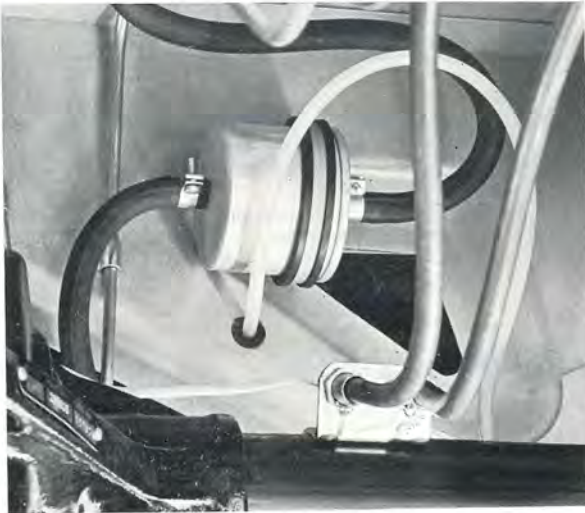
Fig. 2-102. Fuel filter installed
