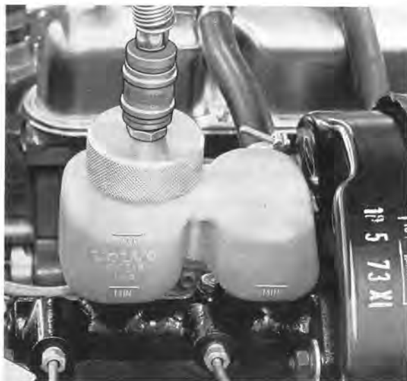
Fig. 5-61. Connecting bleeder unit VOLVO 108 662
