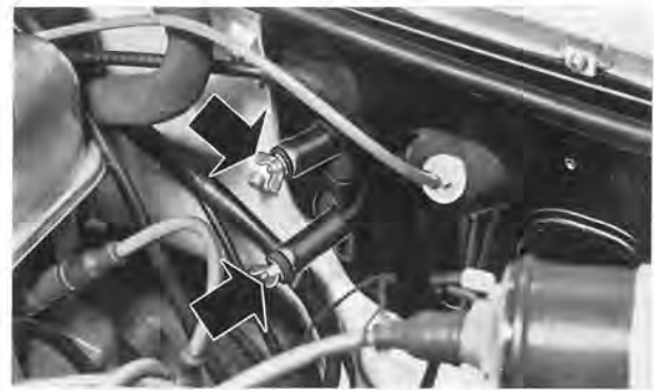
Fig. 8-66. Fitting plugs in heater system connection pipe
