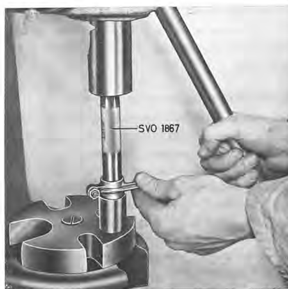
Fig. 2-29. Replacing bush in rocker arm
