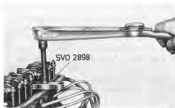
Fig. 2-25. Re-tightening cylinder head bolts
