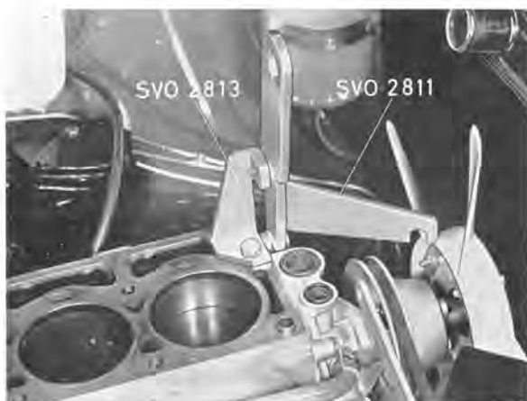
Fig. 2-15. Fitting support 2813 with cylinder head removed
