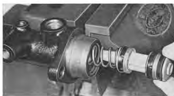
Fig. 5-50. Installing secondary piston
