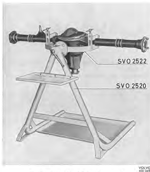
Fig. 4-135. Stand and fixture for rear axle
