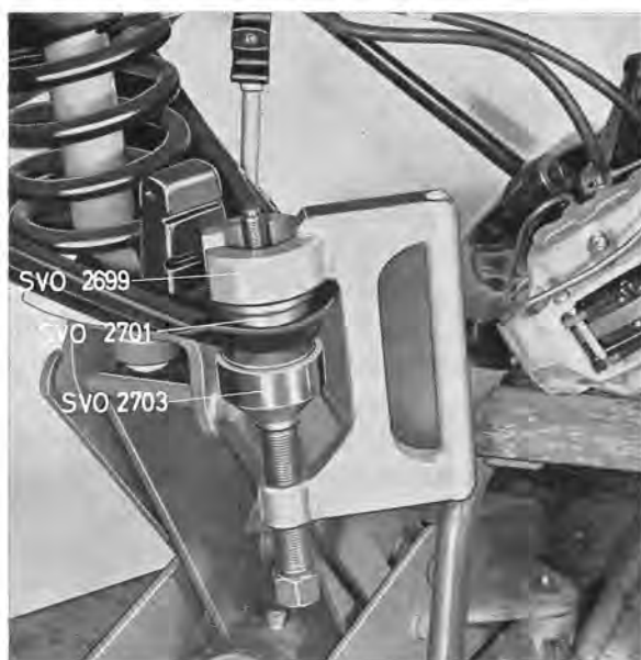
Fig. 6-30. Installing lower ball joint
