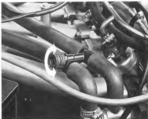
Fig. 2-120. Idle adjusting screw
