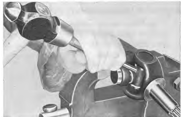
Fig. 4-131. Removing spider, I
