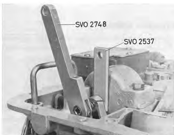
Fig. 4-119. Adjusting front brake band
