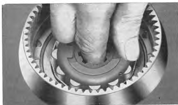
Fig. 4-55. Fitting the uni-directional clutch
