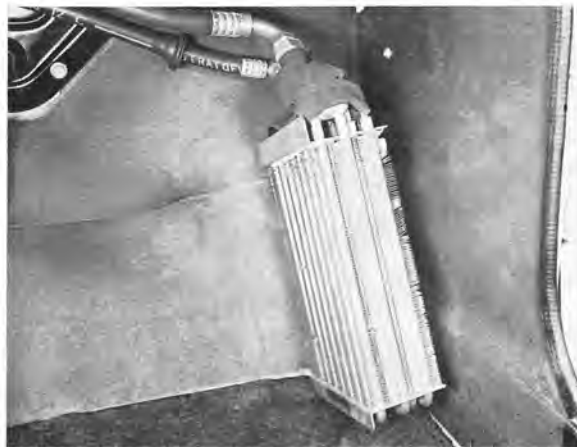
Fig. 8-70. Location of evaporator on floor
