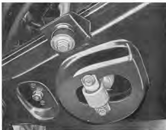
Fig. 7-9. Lower attachment, front shock absorber
