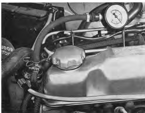
Fig. 2-140. Connecting pressure gauge
