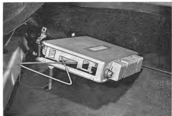
Fig. 2-136. Removing plug contact
