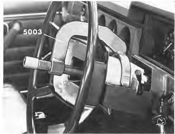
Fig. 6-46. Removing steering wheel
