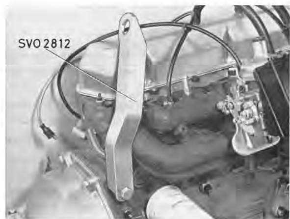
Fig. 2-14. Lifting arm 2812 on rear end of engine
