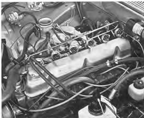
Fig. 2-142. Injectors removed for checking
