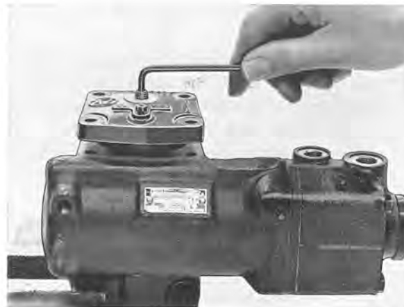
Fig. 6-59. Removing housing cover
