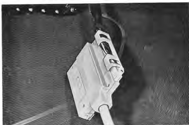
Fig. 2-131. Test instrument connected to cable harness
