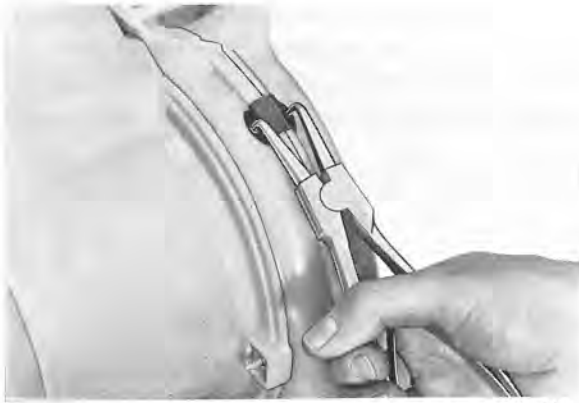
Fig. 8-60. Installing clamps for outer end
