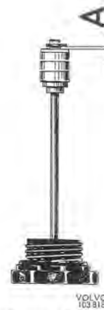
Fig. 2-86. Damper plunger clearance
