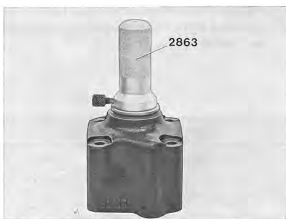
Fig. 6-74. Installing sealing ring
