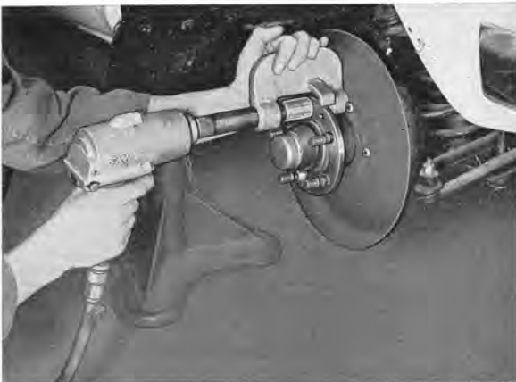
Fig. 7-17. Installing wheel stud
