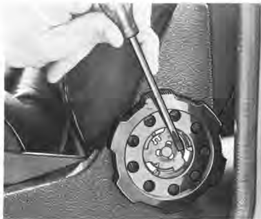
Fig. 8-49. Installing hand wheel
