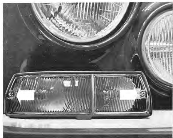
Fig. 3-98. Removing flasher light glass
