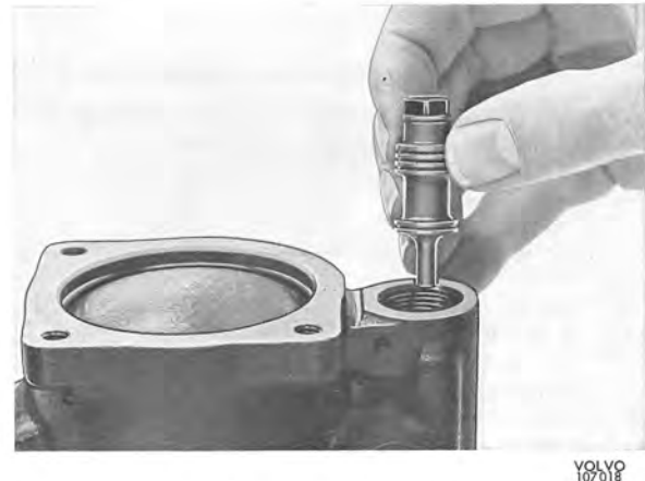
Fig. 6-97. Installing control valve
