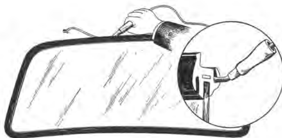
Fig. 8-29. Placing cord in rubber strip
