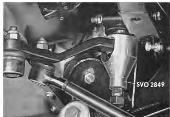
Fig. 6-57. Removing pitman arm
