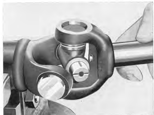
Fig. 4-132. Removing spider, II
