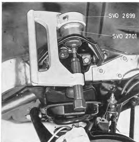
Fig. 6-21. Removing upper ball joint
