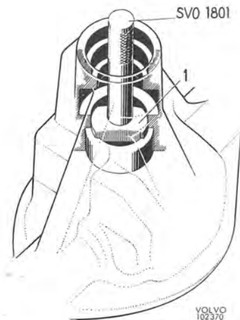
Fig. 4-148. Removing rear pinion bearing race 1. Removing drift 2843
