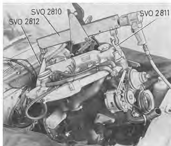
Fig. 2-16. Lifting engine, B 30 E/F
