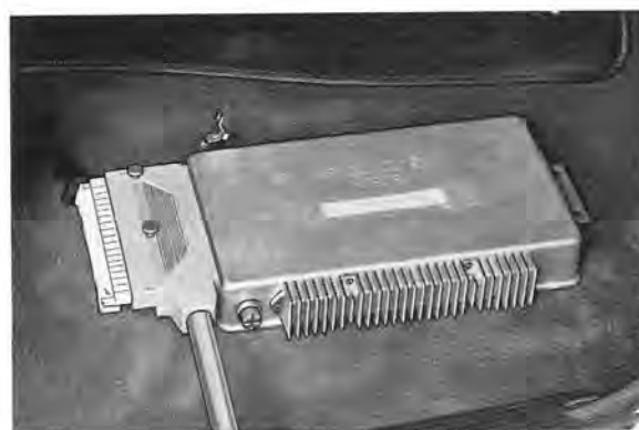
Fig. 2-132. Test instrument connected to cable harness
