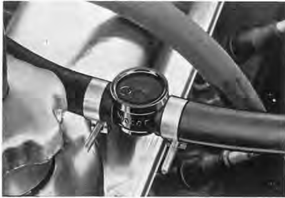
Fig. 5-75. Check valve installed
