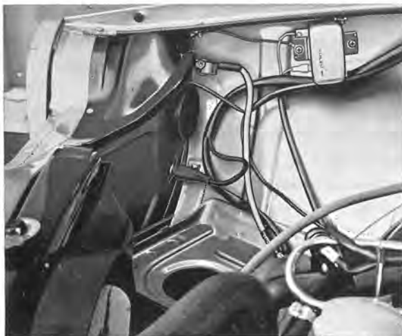
Fig. 2-117. Temperature sensor for intake air, installed
