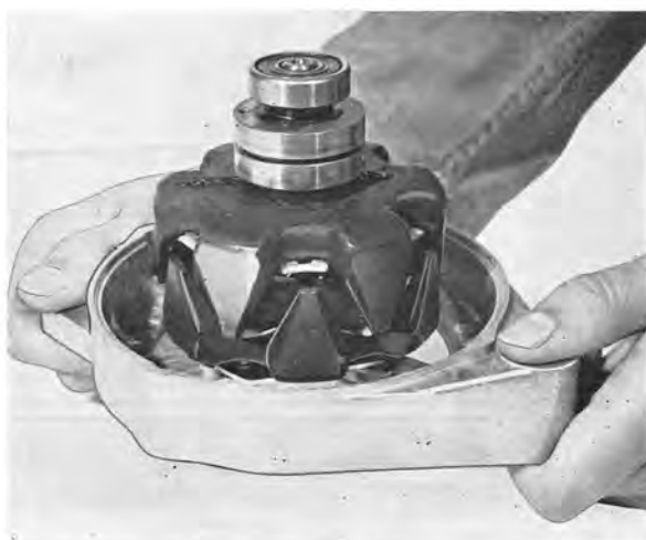
Fig. 3-8. Removing drive end shield
