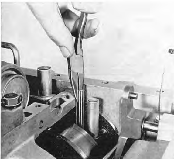
Fig. 4-86. Removing converter inlet and outlet tubes using needle-nose pliers
