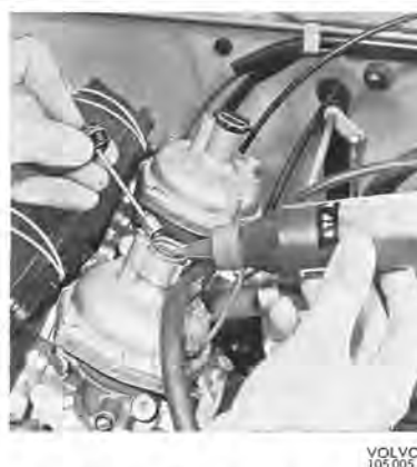
Fig. 1-2. Checking the oil level in centre spindle
