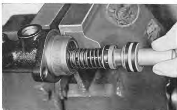
Fig. 5-52. Fitting primary piston
