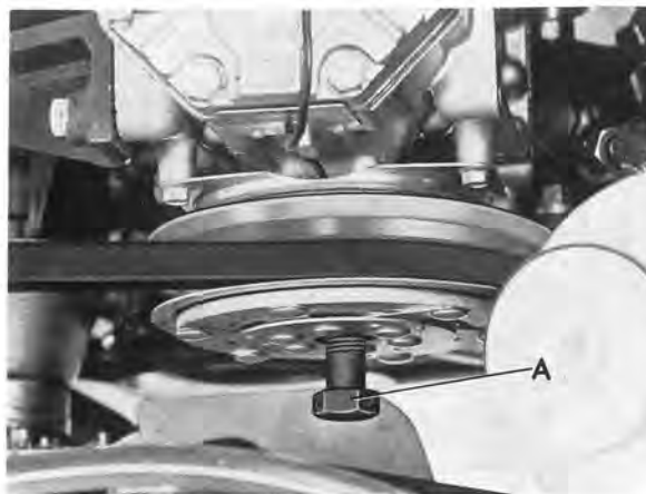
Fig. 8-82. Removing pulley A. Bolt 5/8" UNC
