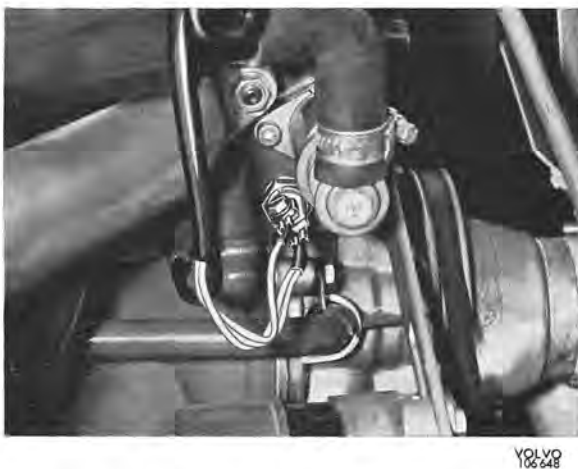
Fig. 2-115. Thermal timer installed
