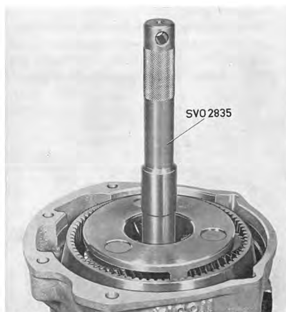
Fig. 4-57. Installing planet gear
