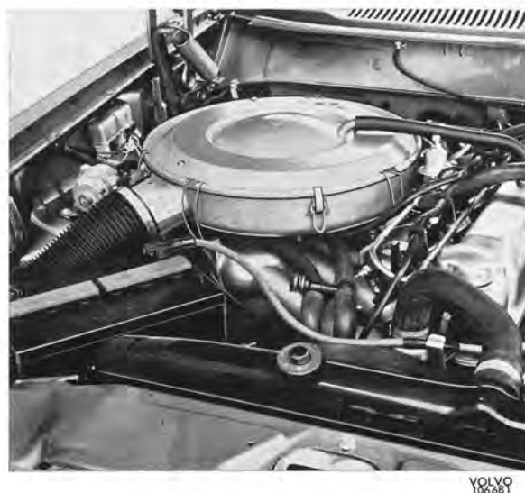
Fig. 2-119. Air cleaner, installed
