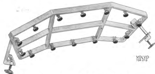
Fig. 8-3. 2899 Fixture for fitting windshield
