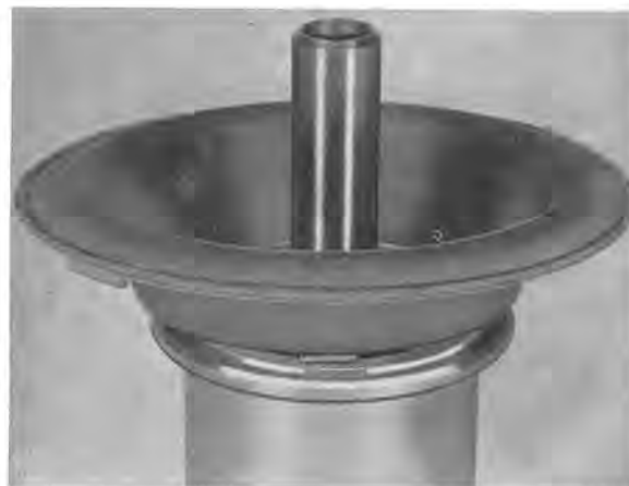
Fig. 2-83. Diaphragm in air valve
