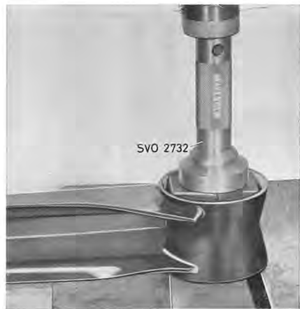
Fig. 7-11. Removing (and installing) the front bush, support arm
