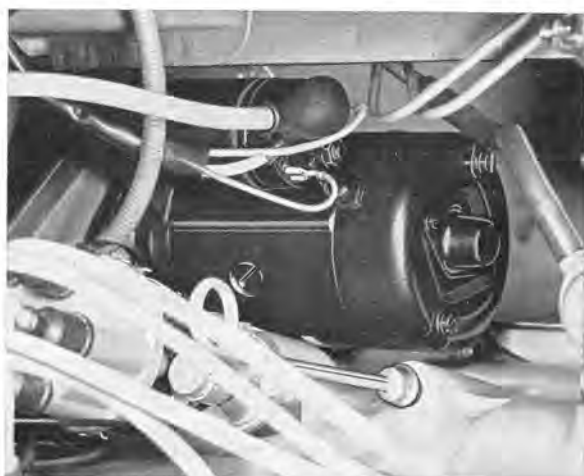
Fig. 3-29. Starter motor installed
