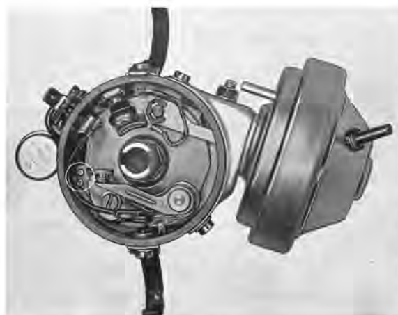
Fig. 3-58. Recess for adjusting ignition contact breaker
