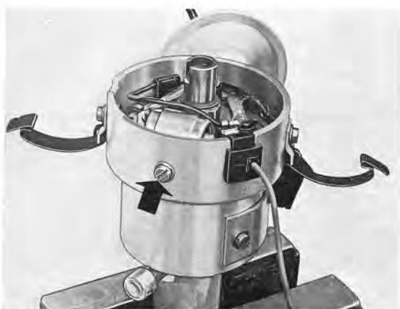
Fig. 3-62. Removing condenser and primary cable
