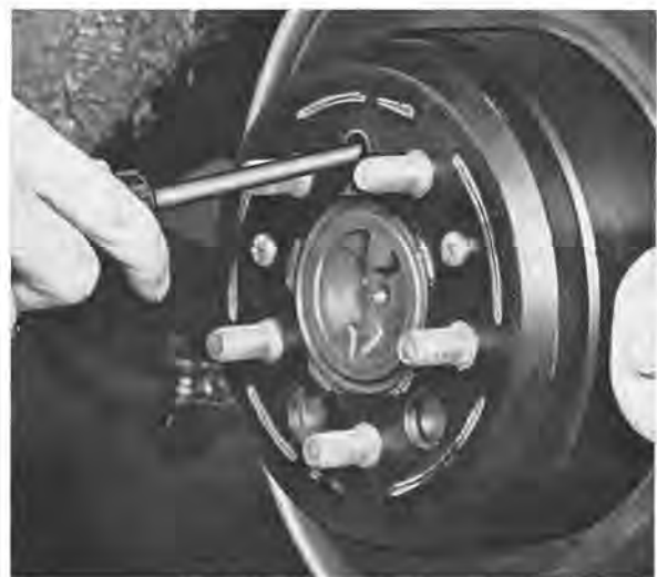
Fig. 5-78. Adjusting the parking brake, rear wheel
