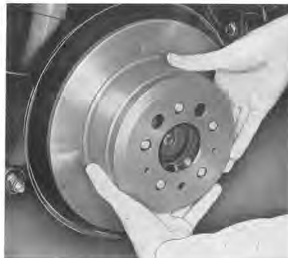
Fig. 5-83. Removing the brake drum
