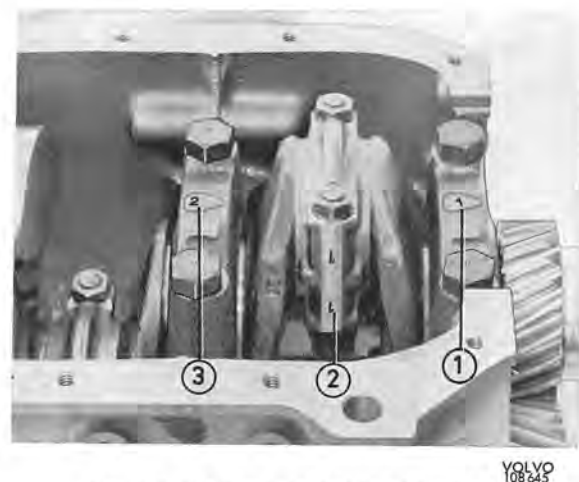
Fig. 2-21. Marking main and big-end bearings 1. Main bearing No. 1 2. Big-end bearing No. 1 3. Main bearing No. 2
