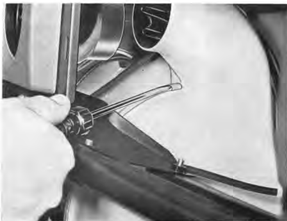
Fig. 8-58. Removing clamps for outer end
