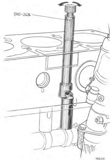
Fig. 2-20. Removing valve tappet
