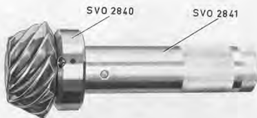
Fig. 4-154. Adjusting ring and tool for pinion location
