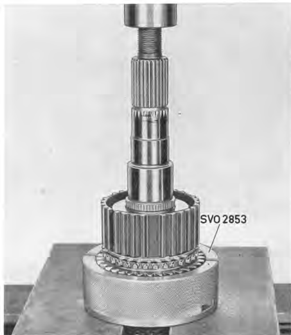
Fig. 4-24. Disassembling mainshaft, I
