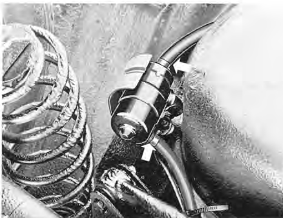
Fig. 2-137. Removing fuel pump
