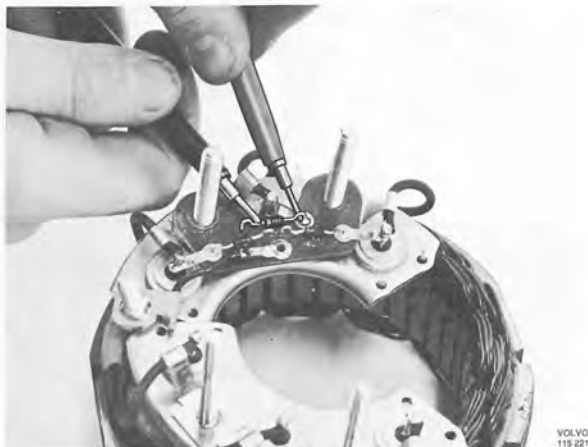
Fig. 3-11. Checking magnetizing diodes
