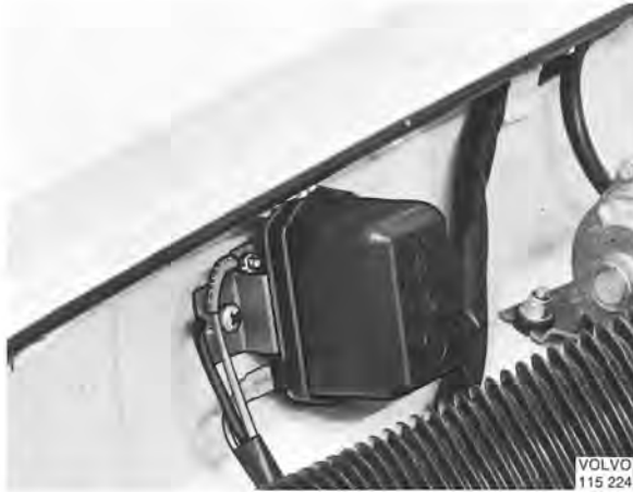
Fig. 3-20. Voltage regulator fitted
