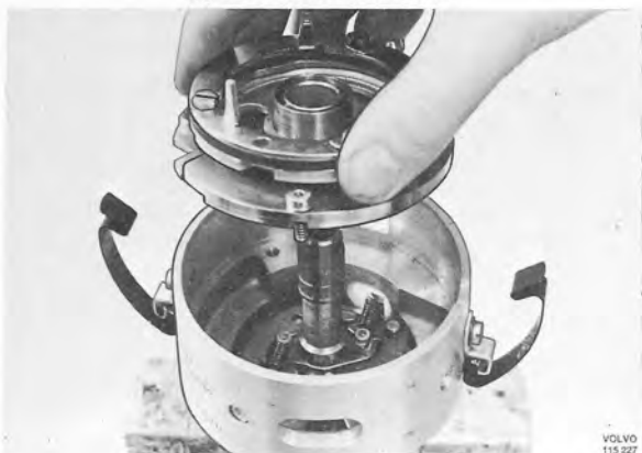
Fig. 3-78. Removing impulse sender
