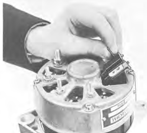
Fig. 3-6. Removing brush holder
