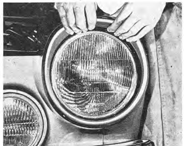
Fig. 3-89. Removing outer rim
