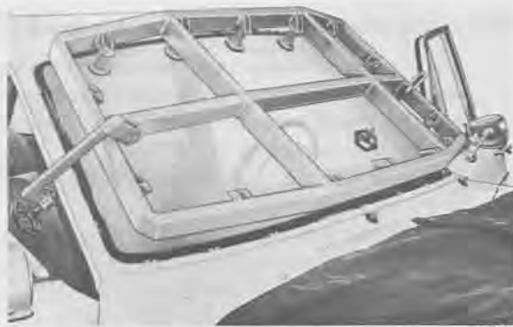
Using fixture 2899 to install windshield
