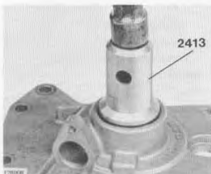
2413 Drift removing/installing rear cover seal
