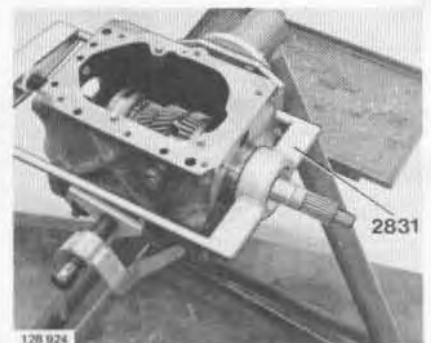
2831 Press tool installing main shaft bearing
