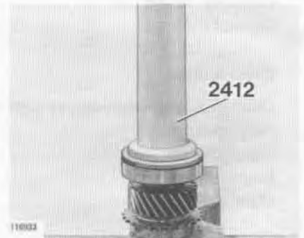
2412 Drift installing input shaft bearing
