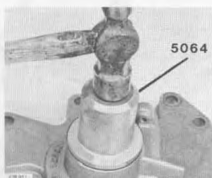
5064 Drift installing rear cover seal
