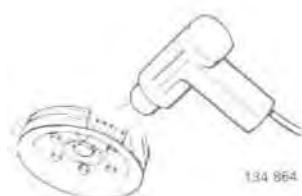
**Check centrifugal advance at 42 r/s (2500 r/min)**
