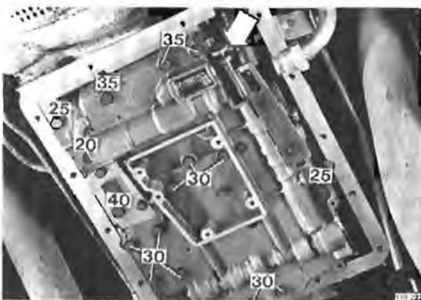
BW55, screw lengths in mm
