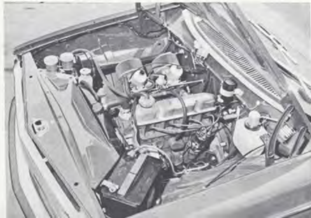
The engine is identical with that of 1800S sports coupé so the carburettors have only paper-element air filters. The brake servo and master cylinders are behind the righthand headlamp with a long push-rod to the pedal
