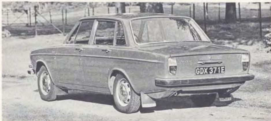
Heavy-duty bumpers have rubber inserts and they just wrap round the corners of the wings. Glass area is generous; there are mudflaps and towing hooks
