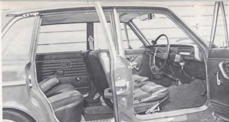
All doors have burst-proof locks and there are rubbing strips over the door sills. Backrests are high and the seats quite low with many adjustments
