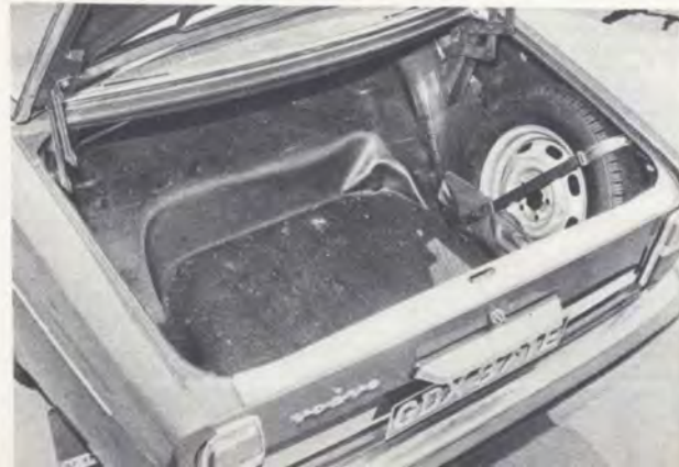
The boot has a moulded rubber mat and a strap to secure the spare wheel and tools. The lid is self-supporting, but the sill is very high
