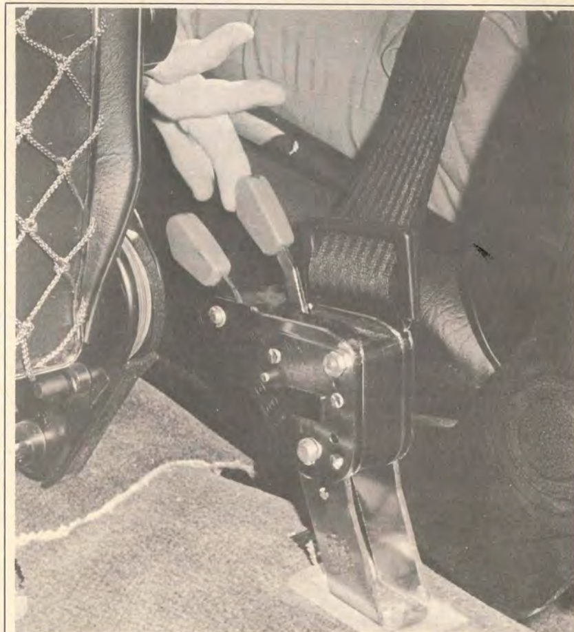
Fingertip release flips Volvo belt tongue out of centre mounting block. System is well ahead of most current standard equipment restraint systems.
