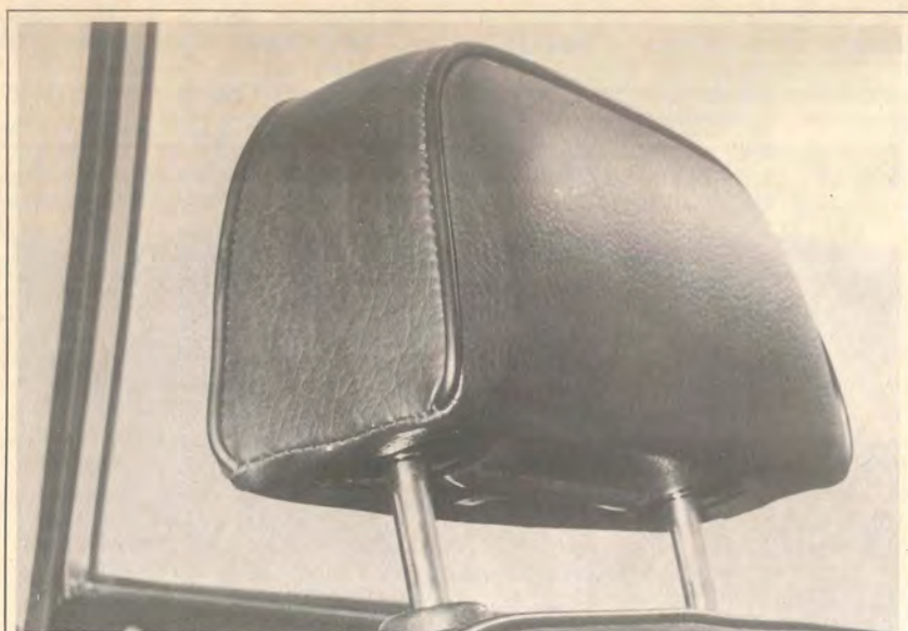
Head restraints are not integral, but are nonetheless properly positioned and adjustable. However, unless locked in place they might fly loose in crash.
