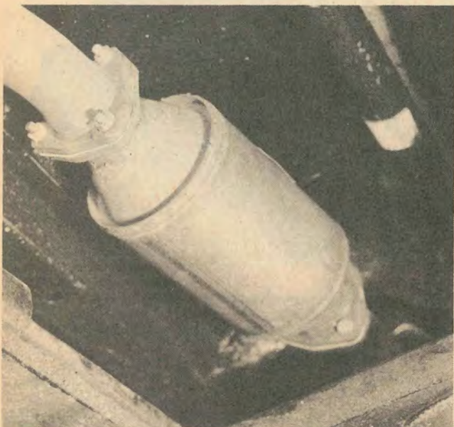
A catalytic converter is used on all California cars, but not in the other forty-nine states. Three bolt flanges allow quick replacement. Cavernous 240 trunk has standup room for the spare and can gobble up suitcases, briefcases and camera gear with room to spare.
