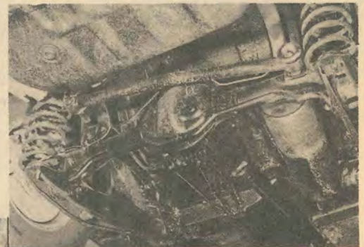
Above, the GL's are all fitted with a Laycock de Normanville overdrive which is operated by a switch on the stick shift when the transmission is in fourth. Large sheetmetal shield under the front of the engine keeps out dirt and big rocks, apart from stiffening up the front end and improving the cooling. Below, a hefty Panhard rod controls the rear axle side motions and prevents any overshoot on turns. Bottom, the small electric fuel pump picks up at the rear of the tank and feeds the fuel injection system. Two rubber mounts provide the sound insulation.
