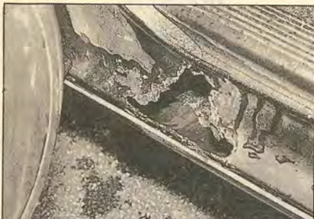
Volvo intended that hot air passing through the sills would drive out moisture and prevent corrosion. It often didn't work...
