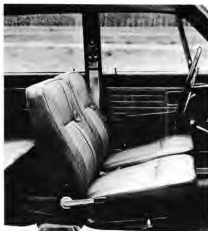
Front seats have infinitely variable backrest angle, fore and aft positioning, plus adjustable stiffness in the critical lumbar region.
